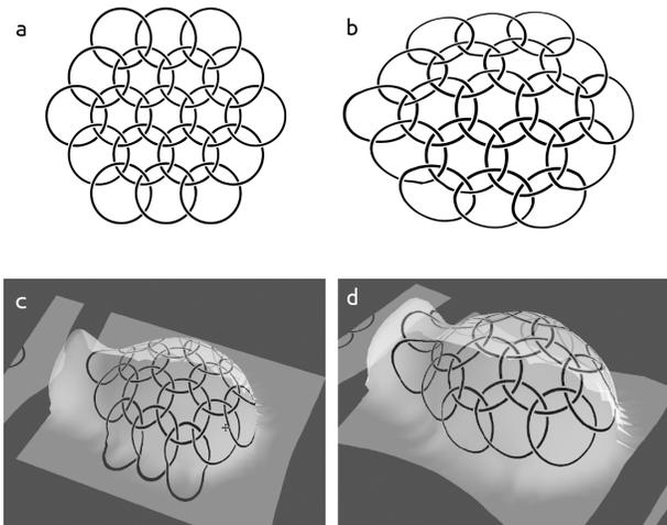
**Figure 6: a: Input un-distorted texture. b: Pre-distorted texture from our pipeline. c: Un-distorted texture mapped onto the 3D shape from vacuum forming. d: Pre-distorted texture mapped onto the 3D shape from vacuum forming.**
