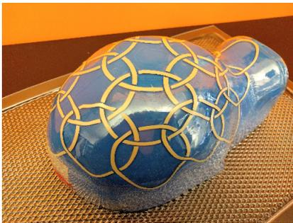
**Figure 7: The physical result of vacuum forming the pre-distorted texture seen in Figure 6b. Although imperfect due to manual manufacturing practice, the peripheral coils are more circular and less distorted than results of un-distorted textures in Figure 2.**
